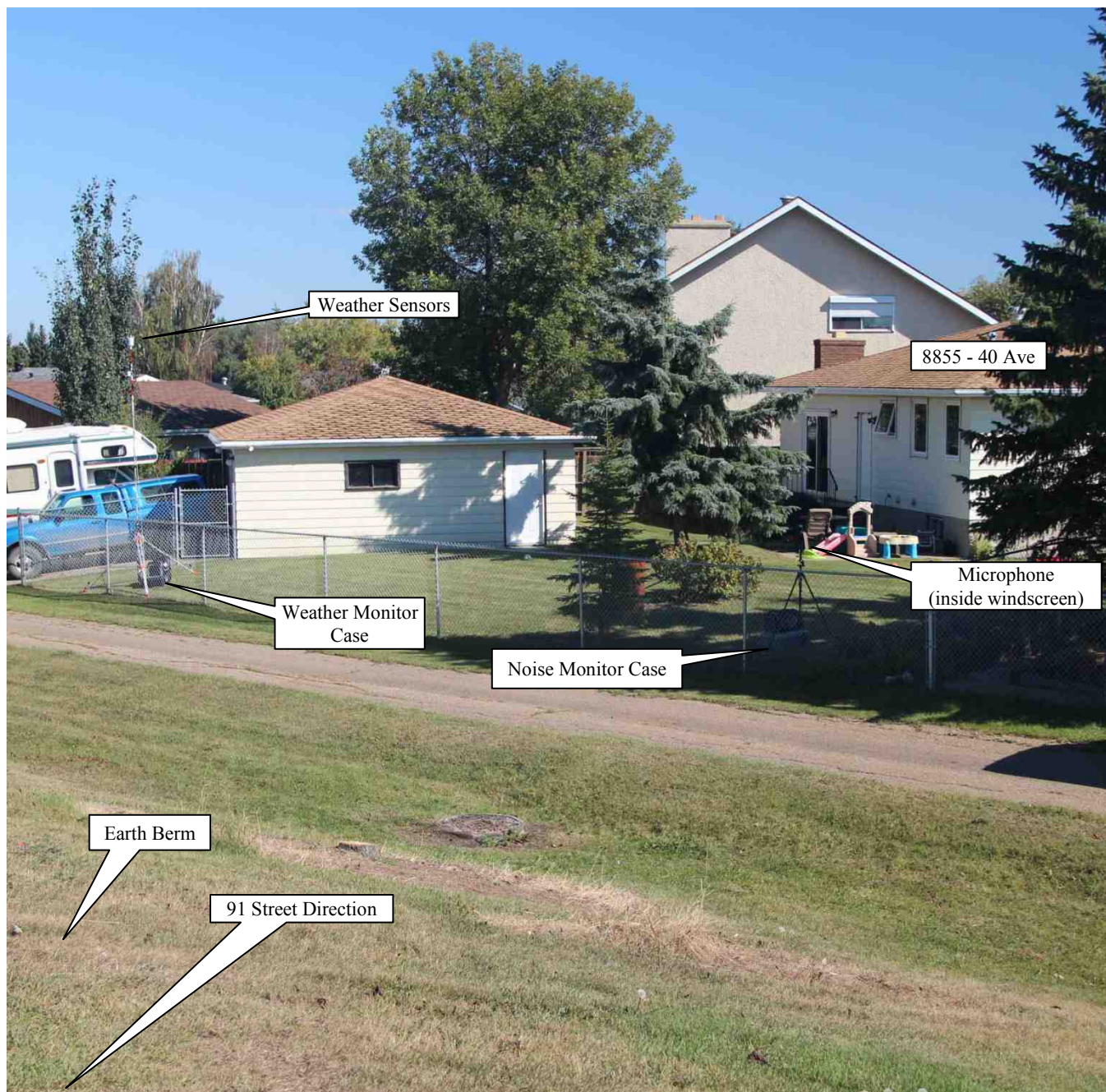
Figure 4. Picture of Noise Monitor at 8855 - 40 Avenue (Fall, 2014)
